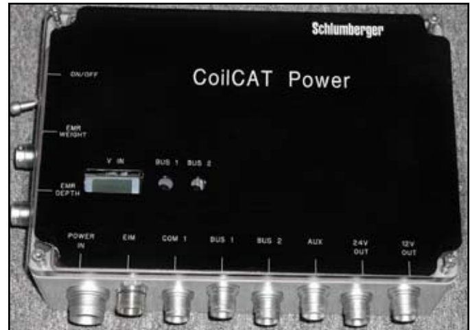
Figure 9-12. Sensor Power Supply
