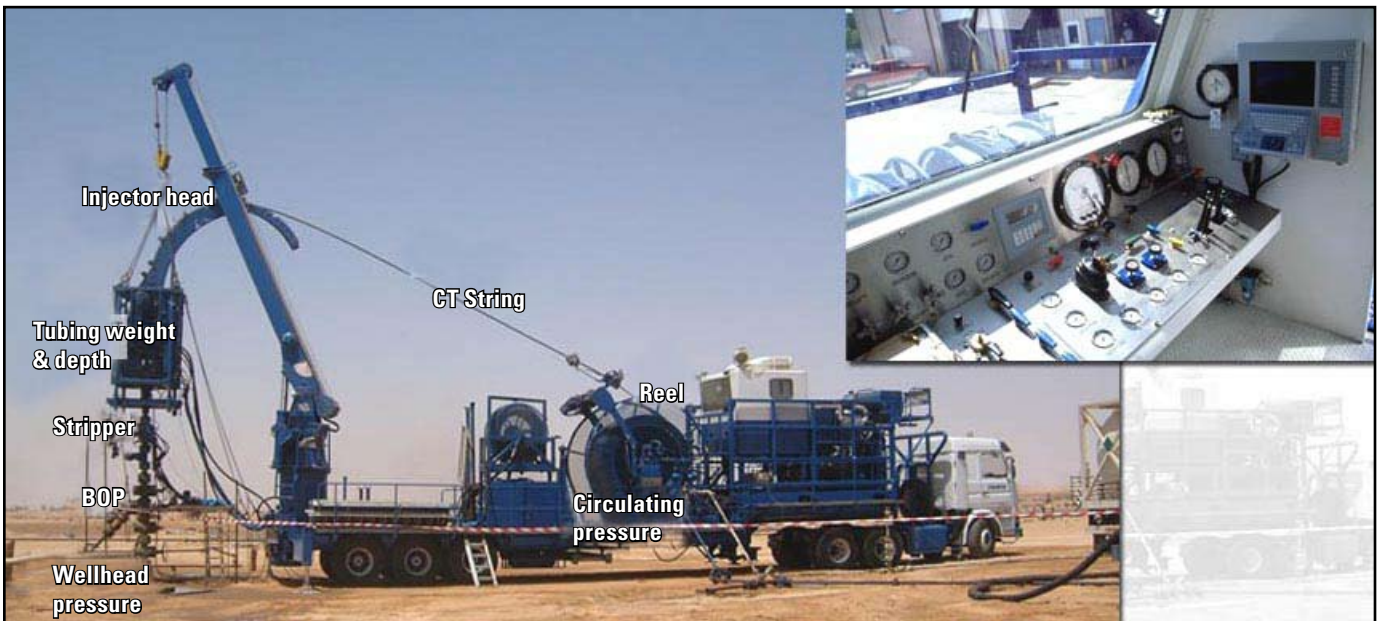
Figure 5-3. Control Console Gauges for Principal Operating Parameters
