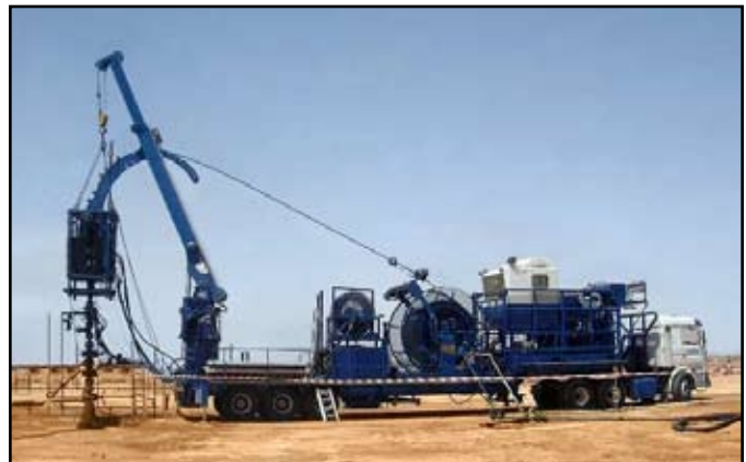
Figure 3-1. Paved Road Trailer-Based CTU
